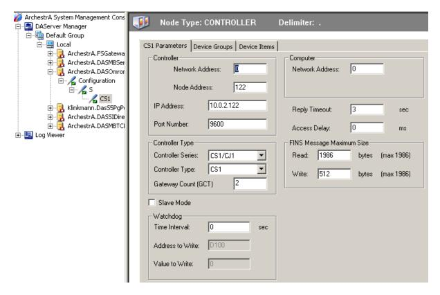
This configuration view has 15 parameters (configuration requires proven network information, it can not be validated by the DAServer):
